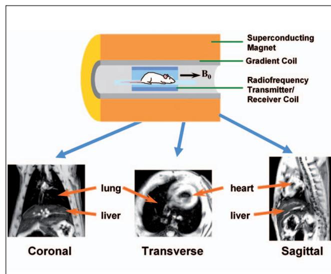
**Fig. 1: MRI equipment for small rodent imaging.**
