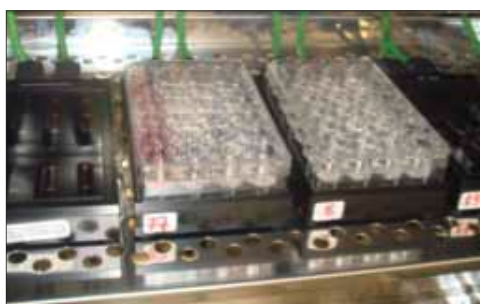
Figure 2. SensorDish reader with OxoDish (A). Setup of multiple OxoDishes connected in series in a humidified cell culture incubator (B). A 96-well Oxoplate (C).
