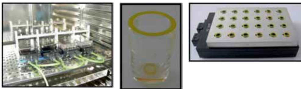
Figure 3. The Sensor Dish Reader (SDR) system from partner PreSens GmbH. This optical fluorescence-based sensor technology allows for optical on-line respiration measurements and monitoring of pH in the cell cultures. Monitoring of the important physiological parameters pH and oxygen is essential for assessing the physiological condition of a cell culture. Consequently, this also becomes an efficient means for detection of toxic effects on the culture. Optical micro-sensors for pH and oxygen offer many advantages over other sensor systems, such as non-invasive and non-destructive measurement from the outside, through the transparent wall of a small bioreactor or cell culture plate. Optical sensors can also easily be combined with other biosensor methods. The panels show culture plates placed in a cell culture incubator for on-line monitoring; one unit of culture well with fluorescence spot; SDR plate optimised for reduced size wells.
